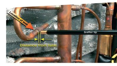
Leak rate signal for leak on backside of a 6 mm (0.25 in) tube joint, leak size  $1 \times 10^{-4}$  mbar l/s (i.e. 22 g/a R134a)
