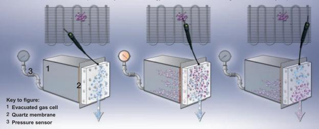
The quartz membrane only has permeability for helium. If helium is detected and is taken in through the sniffer line with air, only the helium fraction penetrates through the membrane, and the pressure in the gas cell rises as detected by the pressure sensor. If afterwards only air is pumped through the sensor, helium will escape the gas cell through the membrane, and the pressure in the gas cell decreases quickly.
