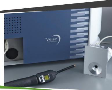
Remote calibrated test leak
